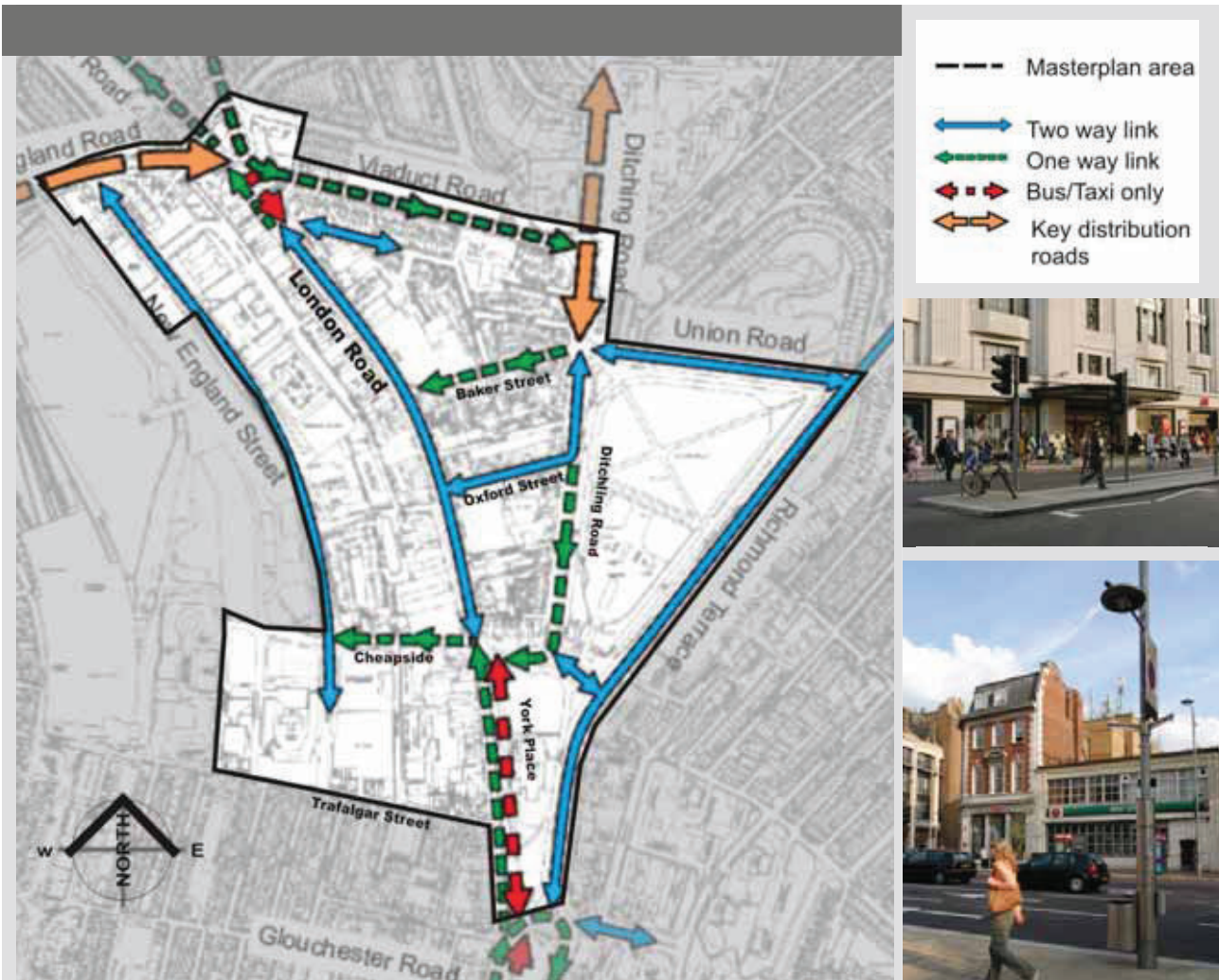
Fig. 6.2: Existing traffic movements: Extract from London Road & Lewes Road Regeneration Strategy's movement vision for the London Road Central area.
